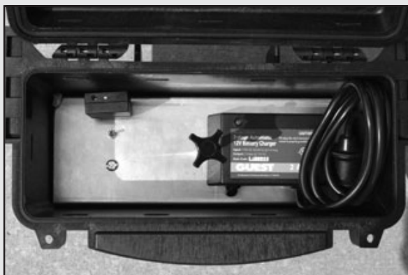
Internal view of SpeedSpy, including EZ Stat, power supply and protected K-band antenna.
